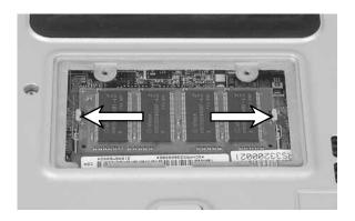
**10** Pull the memory module out of the slot.
